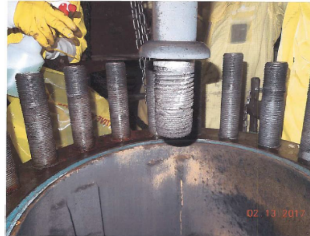
LaSalle 2E22-F004 – Upper wedge with internal threads with severe wear degradation, wedge pin was found sheared.
