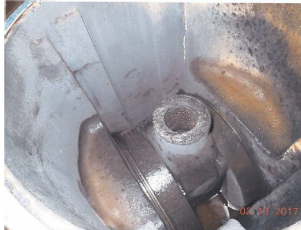
LaSalle 2E22-F004 – Upper wedge with internal threads with severe wear degradation, wedge pin was found sheared.
