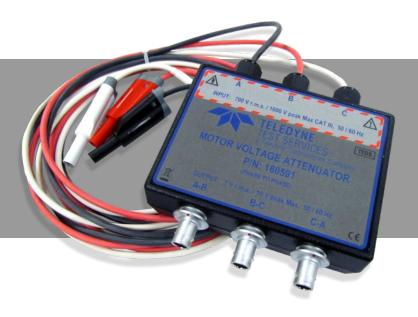
The Teledyne LeCroy Test Services Motor Voltage Attenuator (MVA) products are used to measure motor voltages on 3-phase AC inductive and DC motors. The MVA's use precision attenuators that convert high level AC/DC voltage to low level signals that can be input to the QL3-FS system.
